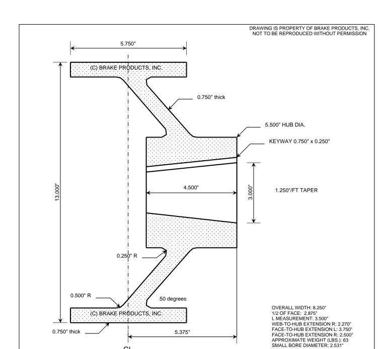
TOLERANCES: WHEEL DIAMETER: +0.005"/-0.000" BORE TAPER: +0.000"/-0.003"
